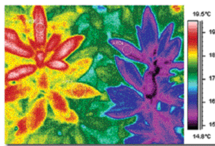
Fig. 1. The thermal radiation emitted from the leaves is detected to demonstrate water stress stress (leaves on the left).
